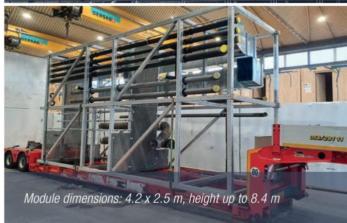
*Module dimensions: 4.2 x 2.5 m, height up to 8.4 m*
